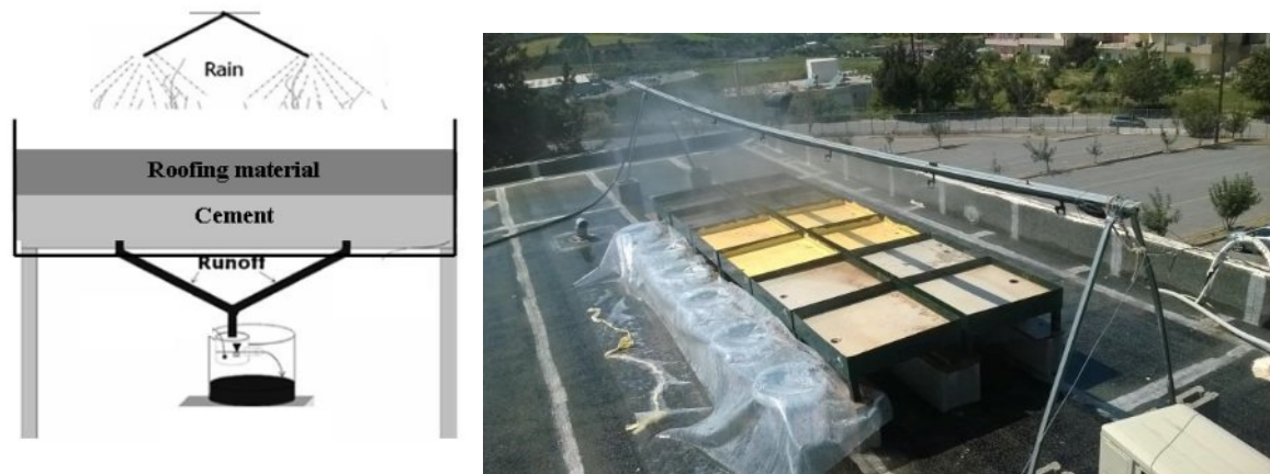
Figure 1. Schematic diagram and general view of lab-scale roof
